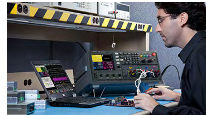
Figure 2 The Keysight N6705C DC Power Analyzer, outfitted with a Keysight N6781A Battery Drain Analyzer module and BV9201B PathWave BenchVue Advanced Power Control and Analysis Software, provides a complete instrumentation solution for performing battery rundown tests.
