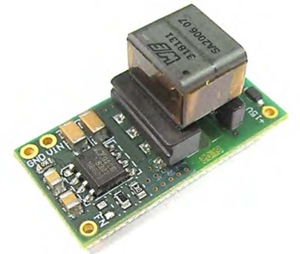
Figure 5 : Würth Elektronik reference design for a compact, isolated DC/DC converter for HV SiC/IGBT Gate Driver.
